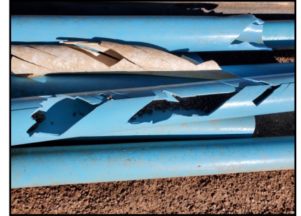
This is what a cold winter without snow does to the water mains .
